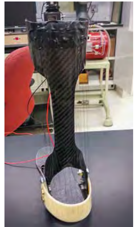
Early prototype for the drop foot push off device
